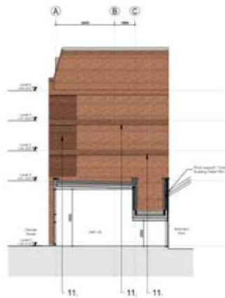
02 - Section through Leeming House connection - Looking East
